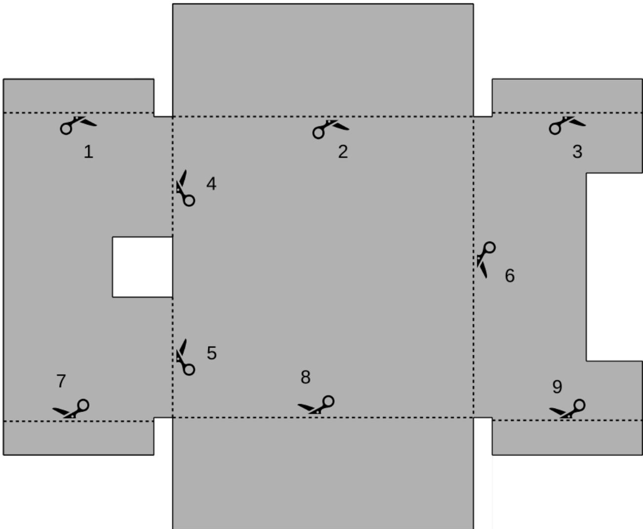
It is sufficient to make a single clean shallow cut along each of the bending lines - you should merely scrape the material, not cut through it.
