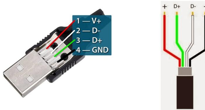
Green and white leads (i.e. the two inner contacts in the USB connector) are used for transferring data and for signaling to the charger that the connected device requires its full power. Signaling is performed simply by short-circuiting those two leads together.
