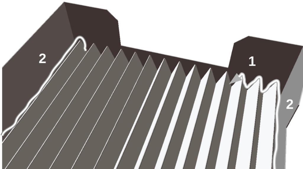
This is the crucial step in making the device. If there are any openings left between the filter material and box walls, the surrounding air would have little reason to flow through the filter material and get cleaned. Such device would be very inefficient in operation.
