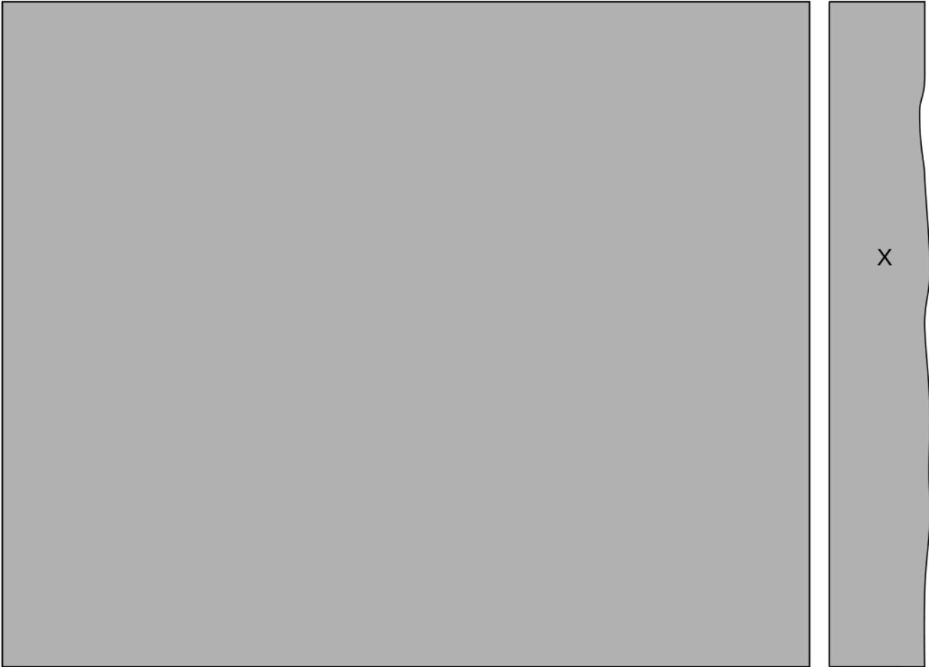
If you have a filter pack consisting of two halves (each 20 cm wide), you will cut out a 40 x 5 cm rectangle from X and use it as a girder put between the halves.
