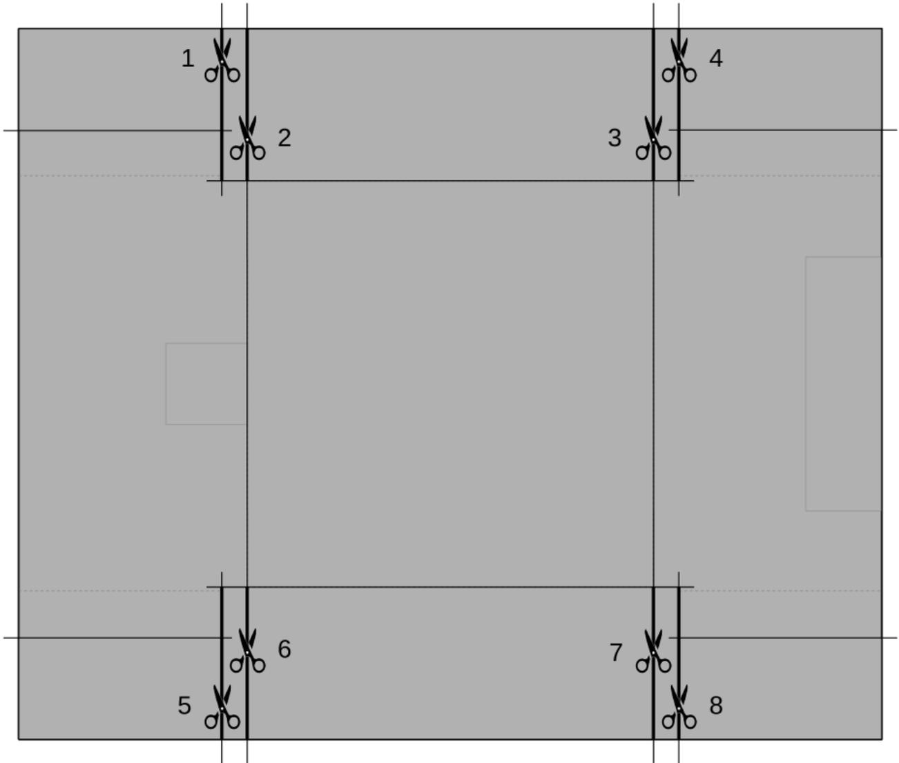
Take care not to cut too much material in the central part of the cardboard – do not cut any further than the crossing lines. This is easiest to prevent by cutting the cardboard starting from center and pulling the cutter towards the edge.
