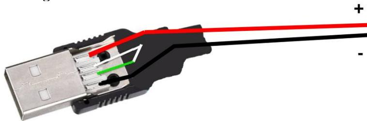
Close the connector and wrap it up with some electrical tape if necessary.
