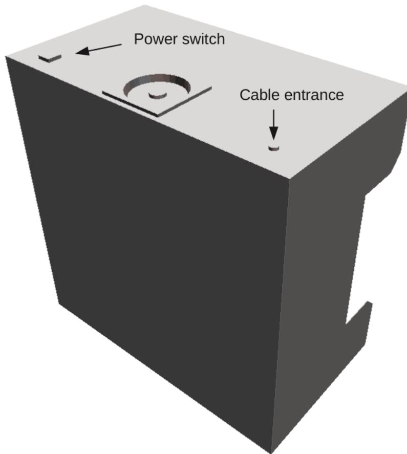
Make the two appropriately sized holes in the cardboard wall.
