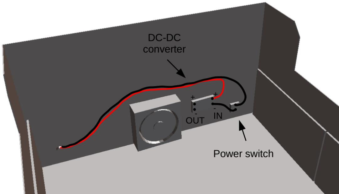
Put the input side of the DC-DC converter circuit board towards the switch.
