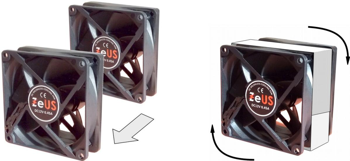
Firmly attach the fans to each other using no less than three full turns of electrical tape.
